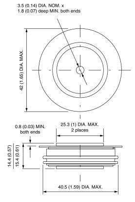
Quote between upper and lower pole pieces has to be considered after application of mounting force (see Thermal and Mechanical Specifications)
